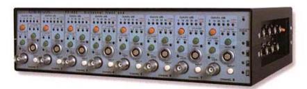
The FC-822 front-end is indispensable for accurate multi-channel sound level measurements. The FC-822 is equipped with eight independent input channels, each one making it possible to select a polarised 200 V microphone or an accelerometer with ICP. regulate gain in 10dB-steps, and insert high-pass and low-pass filters. Each channel has an independent overload indicator.
